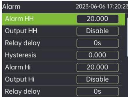
Figure 12 Alarm setting interface
