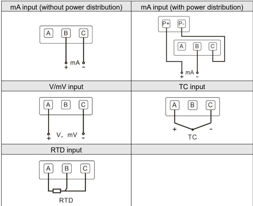
Figure 7 Schematic diagram of signal cable
