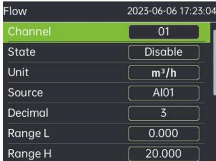
Figure 18 Flow setting interface
