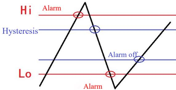
Figure 11 High- or low-level alarm and Hysteresis
