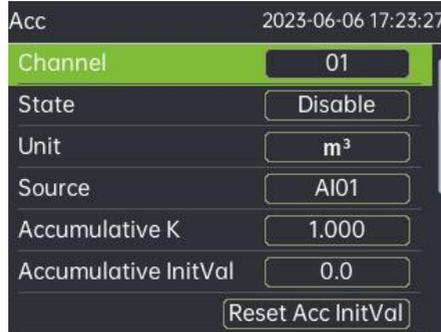
Figure 19 Accumulation setting interface
